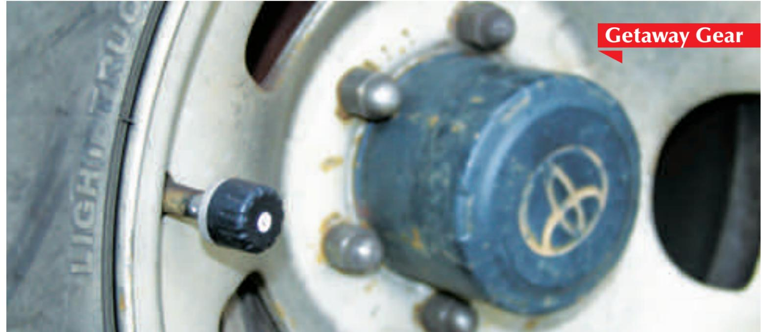
sensors screw onto the tyres' valve stems, constantly monitoring the pressure of the air inside the tyre and sending the information back to the monitor inside the cabin of the tow vehicle. The sensors employ a small hex screw (tool included) to 'lock' onto the valve stem.
